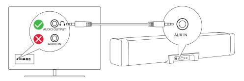
Step 2: Switching the Soundbar to AUX Mode
